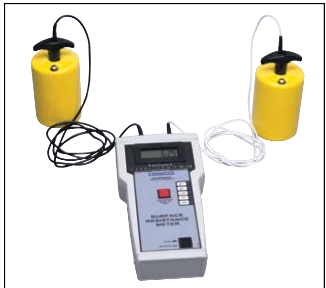
Figure 11. 19780 set up to test resistance point to point
