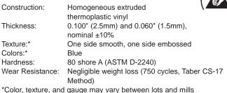
Grounding: This material must be properly grounded for optimum electrial performance. Ask for Technical Brief PS-2013 for mat grounding instructions.
