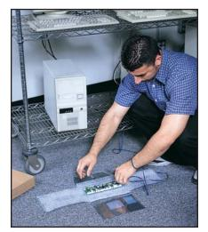
Attached to package is grounding strap with loop on one end to be snugly attached to worker's wrist. Other end has alligator clip to use to ground both worksurface and worker. The Statshield<sup>®</sup> ESD Workstation Pouch provides protective packaging, is a reusable form of RFI and ESD protection, and opens up flat to become an ESD worksurface complete with grounding strap to ground worker and worksurface.
