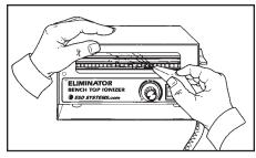
Figure 5. Cleaning the electrodes (Method 2).
