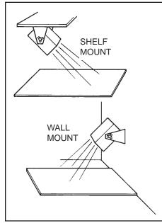
Figure 3. Wall or shelf mounting of the ionizer.
