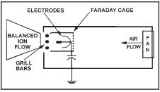
Figure 8. Components of the Faraday Balance System.
