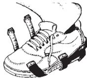
2. Place cup of sole grounder onto the shoe so that the lined cup surface is making contact with the shoe.
