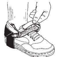
4. Test each heel grounder to confirm proper installation.
