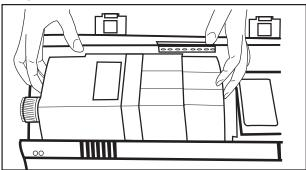
Figure 5: Lifting out the cartridge.
