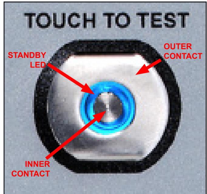
Figure 10. Steady-State Test Switch features and components
