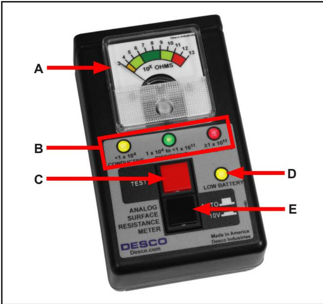
Figure 2. Analog Surface Resistance Meter features and components
