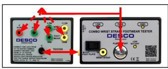
Figure 7. Verifying the calibration of the footwear circuit in the Combo Tester
