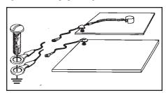
Figure 1. Common point ground for each workstation.
